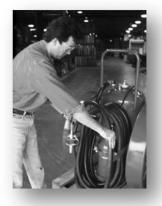
Adjust the loops so that the nozzle fits into the nozzle mount. Loops shall be approximately the same size.
