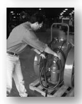
The second loop is a REVERSE loop. Notice that the hose passes behind the loop on this reverse loop. **If instructions are followed, the hose will uncoil without kinks.**
